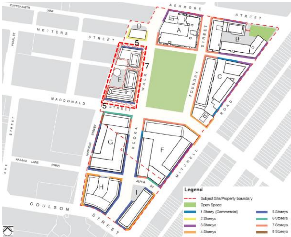
Figure 14: Proposed street wall heights (Block E - outlined by red dashed lines and clouded) - D/2015/966/G
