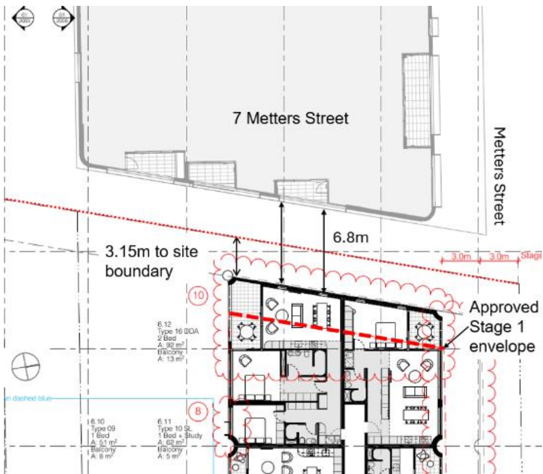
Figure 57: Proposed floor plan at Level 6 of Block E depicting separation to side boundary with 7 Metters Street
